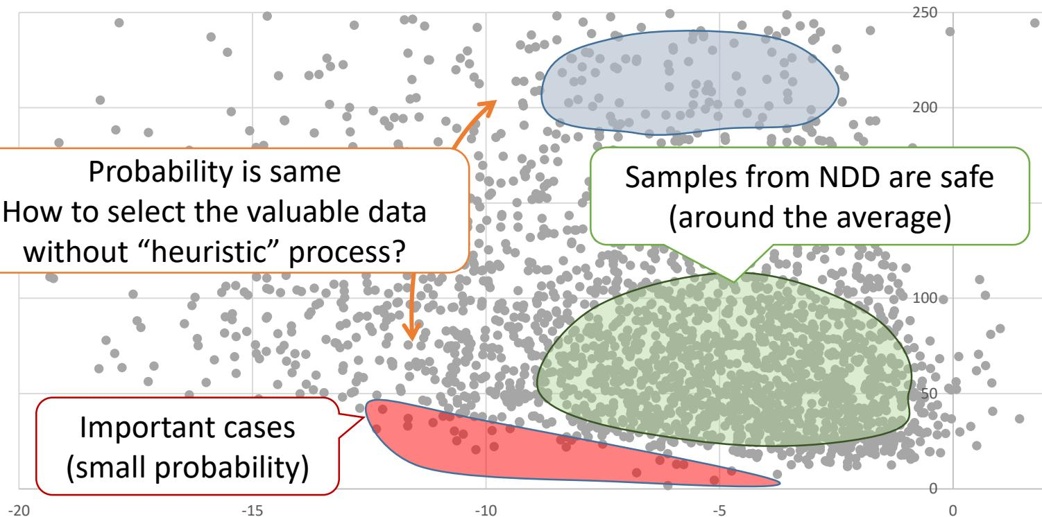
We propose a method to parameter sampling method for test scenarios based on the relationship between the driving parameters and a risk index.
